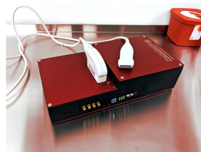
PhotoSound® MoleculUS™, ultrasonic imaging with molecular analysis
