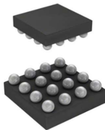
TS8000 Device Size 1.66mm x 1.66mm
