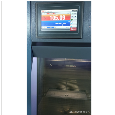
Temperature stress in the climatic chamber
