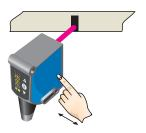
When setting the contrasts to be detected, "1st" flashes. Press set button.
